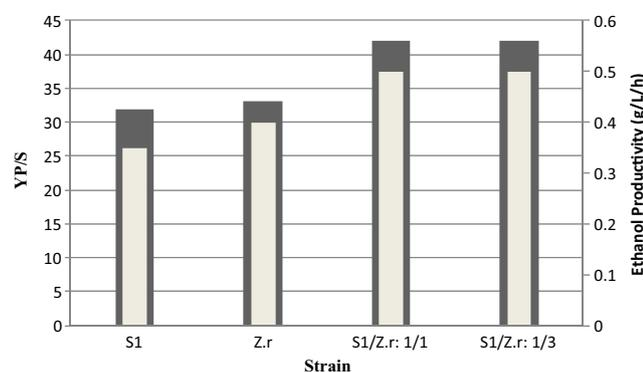
**Fig. 5** Comparison of ethanol production yield (gray bars) and ethanol productivity (white bars) during single cultures of *B. amyloquifaciens* (S1), *Z. rouxii* (Z.r), and their coculture in the ratio S1/Z.r:1/1 and S1/Z.r:1/3 from date syrup with an initial concentration of 400 g L<sup>-1</sup> of total sugars at 150 h of culture
