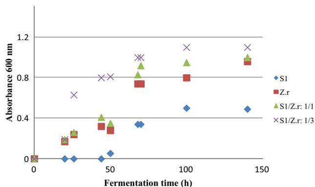
**Fig. 4** Growth of *B. amyloquifaciens* (S1), *Z. rouxii* (Z.r), and their coculture in the ratio S1/Z.r:1/1 and S1/Z.r:1/3 from date syrup with an initial concentration of 400 g L<sup>-1</sup> of total sugars
